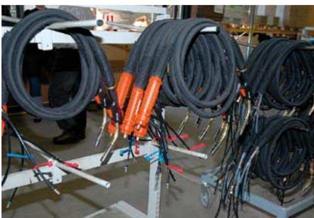
The Kalkkinen factory produces great amounts of air-cooled and water-cooled MIG guns and TIG torches, as well as hundreds of kilometres of cable each year.
